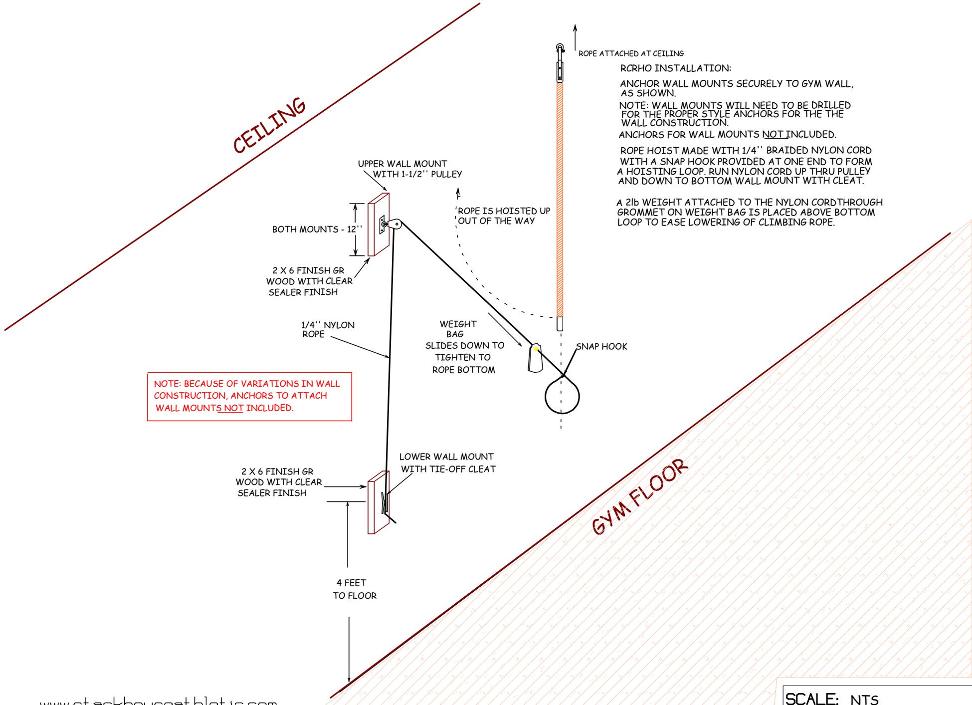
NOTE: BECAUSE OF VARIATIONS IN WALL CONSTRUCTION, ANCHORS TO ATTACH WALL MOUNTS NOT INCLUDED.
